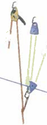
Figure 15-4a: Piggyback with Ratchet in Back
