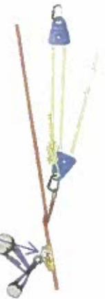
Figure 15-4b: Piggyback with Ratchet in Front
